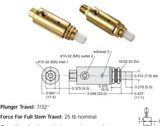
**Operation:** As plunger is depressed pressure increases proportionally to the travel; when plunger is released the input is closed and the output pressure is exhausted to atmosphere
